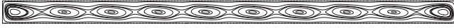
FIG. 7. A typical instantaneous streamline pattern for Le=100 , \psi=0.1 , Ra=28 during the oscillation.
